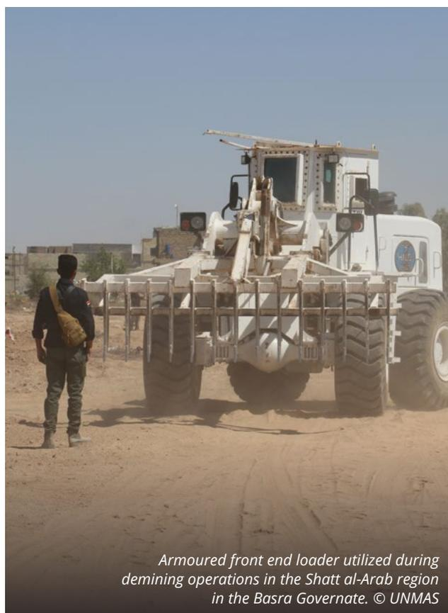
*Armoured front end loader utilized during demining operations in the Shatt al-Arab region in the Basra Governate. © UNMAS*
